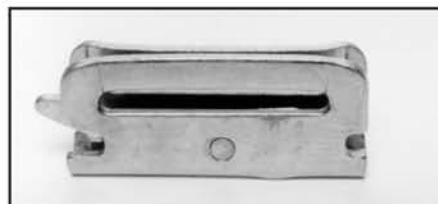
ITEM: 2" Spring E-clip BREAK STRENGTH (lbs.): 3500 W.L.L. (lbs.): 1100
