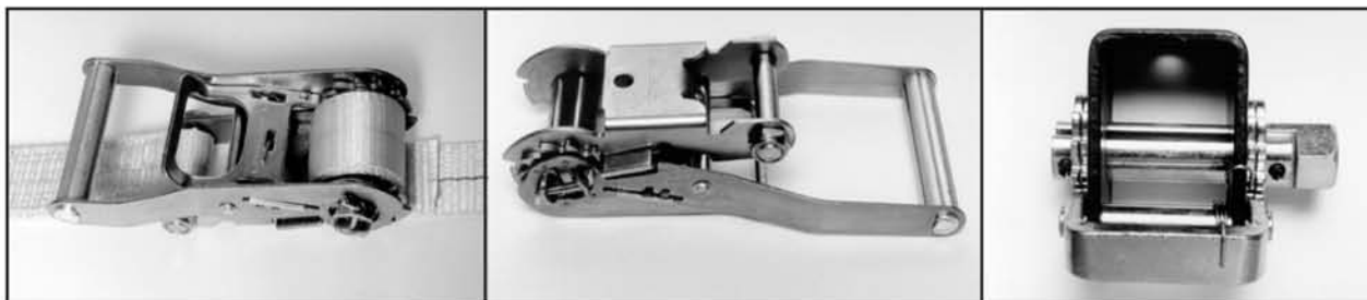
ITEM: 2" Short Wide Ratchet BREAK STRENGTH (lbs.): 10000 W.L.L. (lbs.): 3300
