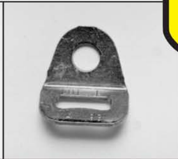
ITEM: Bent Bolt Plate BREAK STRENGTH: 1500 W.L.L. (lbs.): 500
