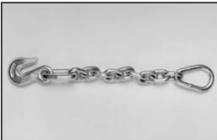
ITEM: Chain Extensions BREAK STRENGTH (lbs.): 16,200 W.L.L. (lbs.): 5400
