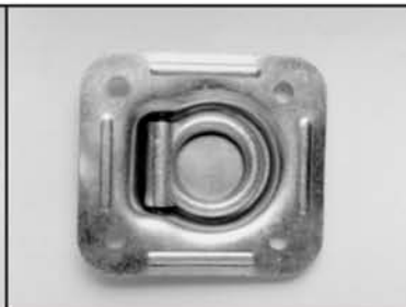
ITEM: Recessed Floor Ring BREAK STRENGTH (lbs.): 5000 W.L.L. (lbs.): 1600
